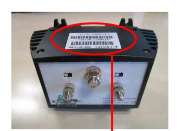
The part and the serial numbers of the appliance are written on the grey label stuck on the top side.
