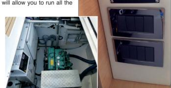
5 : On recent boats, the generator is almost more important than the engines. A powerful generator allows a large battery bank to be recharged in two hours, and limits the noise disturbance.
