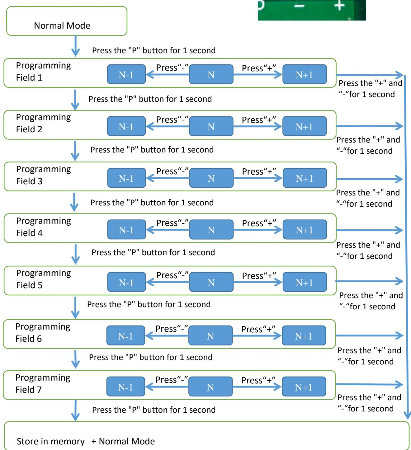
In programming mode, the number of flashes of LED "ON" gives the programming field, the number of flashes of the green LED "FLOATING/REFRESH" gives the programming value.
