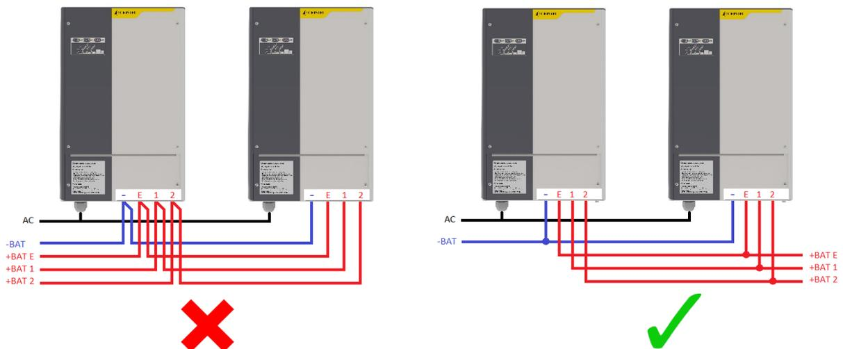
**Step 2 :** **Control wiring :** The parallelization cable links the pin L of connectors X1200 of each charger. A single, insulated, multi-conductor cable, cross-section 1 mm<sup>2</sup> is employed. Its length between the two battery chargers shall not exceed 1 meter.
