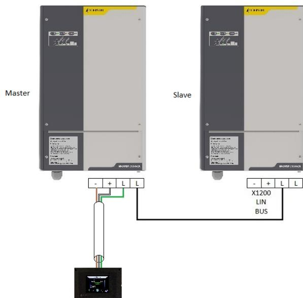
**Case 2 :** When battery chargers with integrated display are installed in parallel, only one display shall operate as Monitor. The others shall operate into Read only mode (Display Setup 2/2 menu). When the monitor goes into stand-by, the Read-only displays will stop emitting information.
