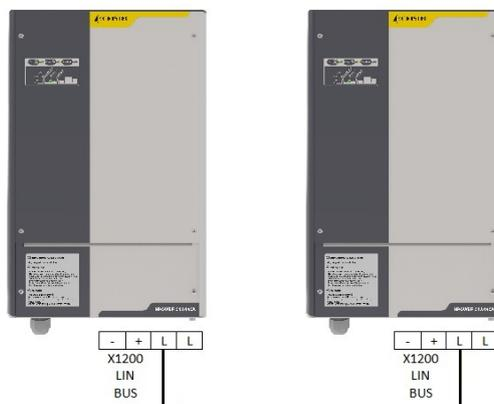
**Etape 3 :** **Select an identifier (ID) per charger :** only one charger shall be Master, ID from 0 to 12. The other is Slave. Its ID shall be n°13, n°14 or n°15 (Switches 1, 2, 3 and 4 – rep. SW1202) :
