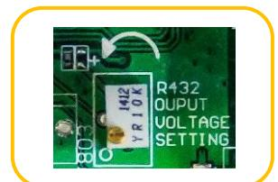
For special batteries, call in a professional installer, who will make the specific settings in accordance with the battery manufacturer's specifications and according to the specifics of the installation.
