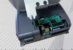
CAN-BUS interface board allows the charger to communicate with a monitoring system or any other peripheral device using this mode of communication. Protocol can be made-to-measure on request.(2)
