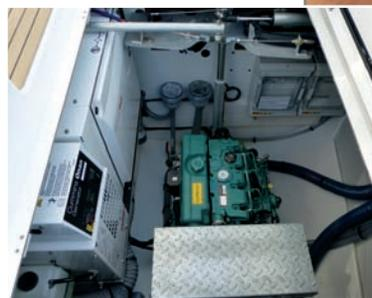
5 : On recent boats, the generator is almost more important than the engines. A powerful generator allows a large battery bank to be recharged in two hours, and limits the noise disturbance.
