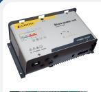
The CRISTEC shore power units combine a battery charger and an electrical panel in a single enclosure. The AC network protection is provided by a 16A/30mA bipolar main circuit breaker and 10A MCB.
