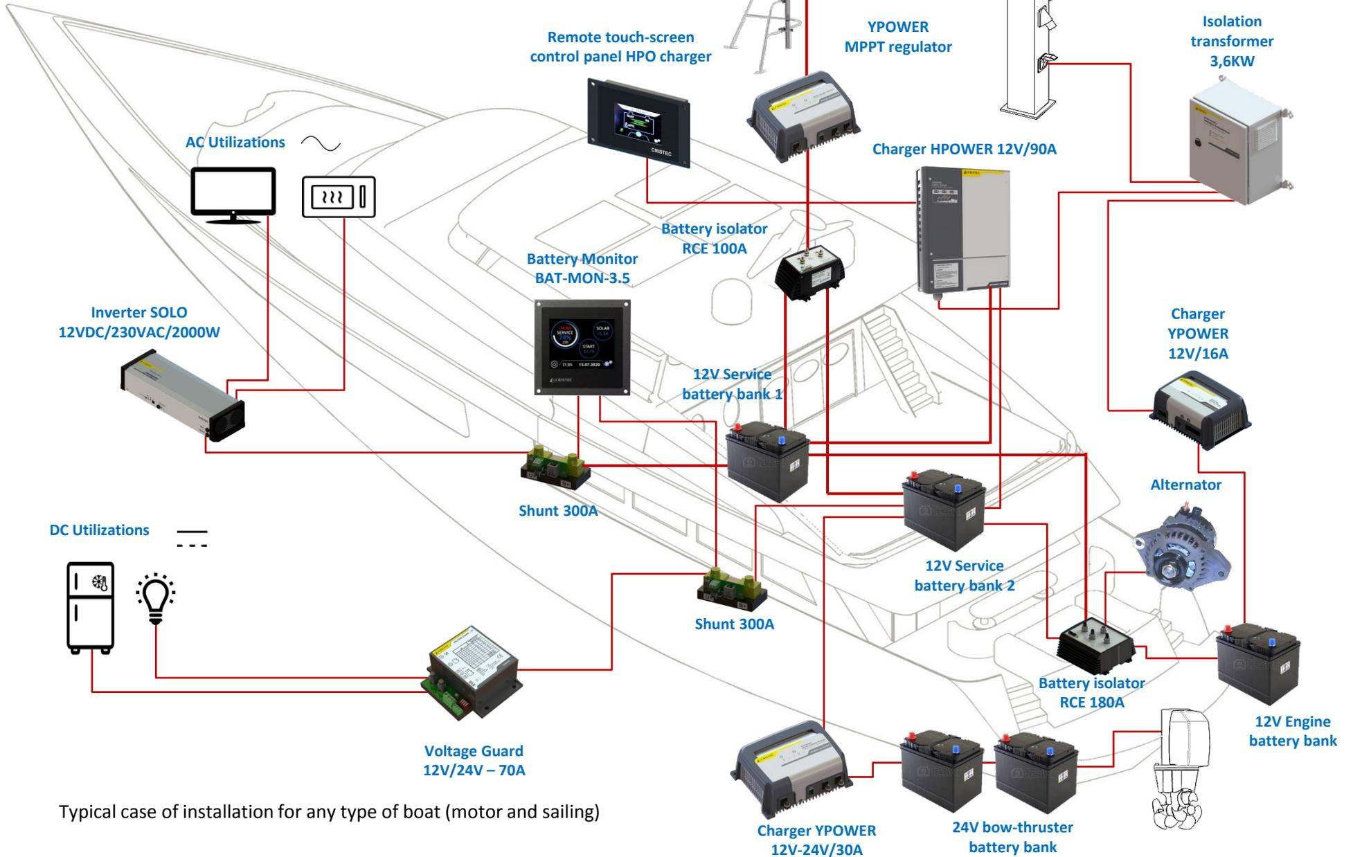
Typical case of installation for any type of boat (motor and sailing)
