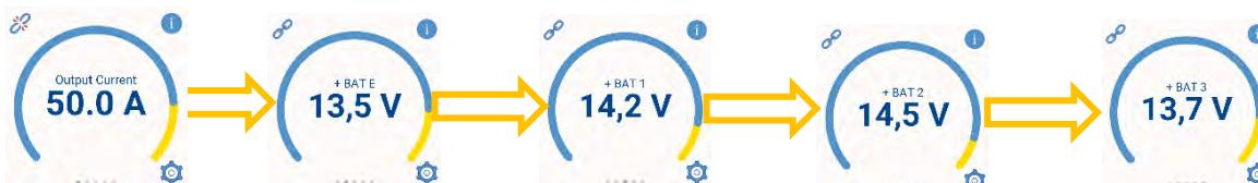
On the lower part, the charging phase information, the voltages and current of the charger, as well as the temperature (with optional probe) and the AC input voltage and frequency.
